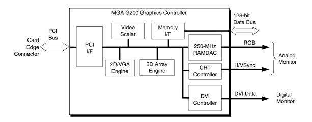
Figure H-3. MGA G200 Graphics Controller Architecture
